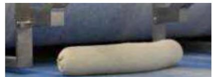
The Rademaker Crusto bread line is capable to handle capacities up to 6.000 kg/hr. The standard Rademaker Crusto bread line can cut 85 strokes/minute, ending up with 10.000 half baguettes or 5.100 long baguettes per hour. Special bread lines can produce up to 30.000 baguettes/hour, at 125 strokes/minute. Rademaker can guarantee an impressive weight accuracy on the baguette production; +/- 2,5 - 3% (+/-5 gram) on the total product weight. An even
